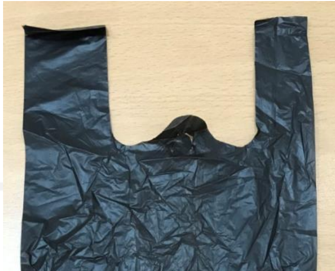
Gambar V.3 Gambar jenis cacat handle misalignment
