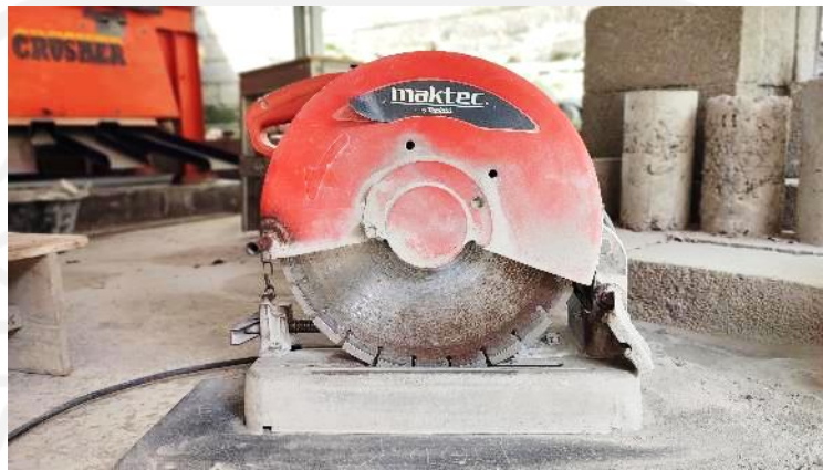
Gambar 4.10 Mesin Pemotong Paving Block
