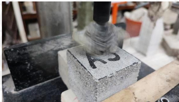
Gambar L-5.2 Proses Pengujian Keausan Paving Block
