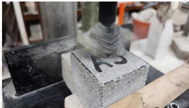
Gambar 5.6 Pengujian Keausan Paving Block
