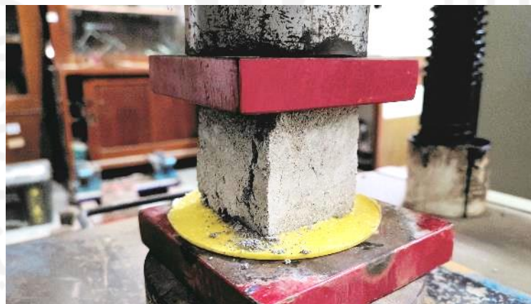
Gambar 5.3 Pengujian Kuat Tekan Paving Block
