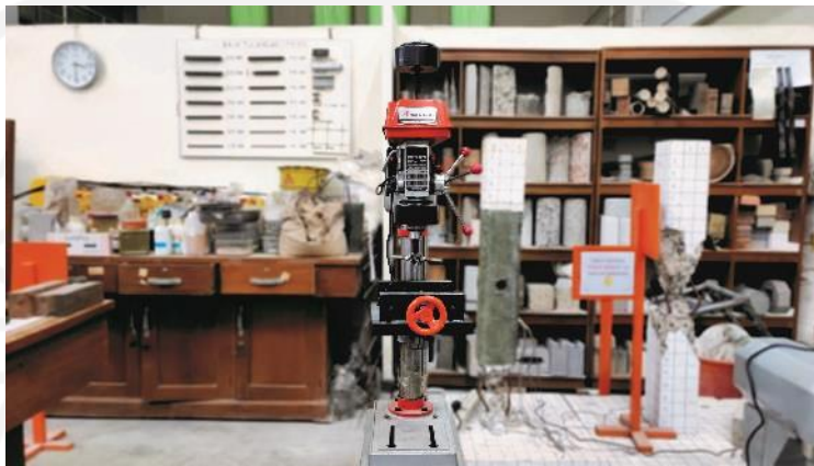
Gambar 4.12 Mesin Uji Keausan Paving Block
