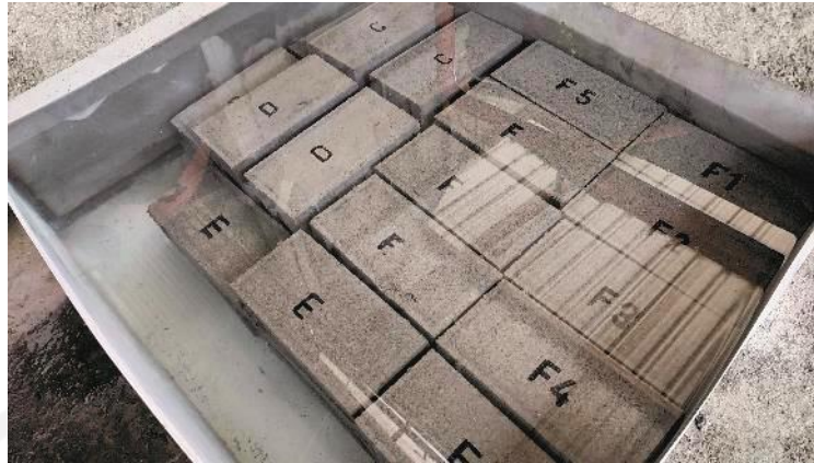
Gambar 4.18 Proses Perawatan Paving Block
