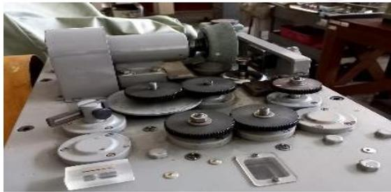
**Gambar 3- 6 Universal Friction Wear Tester**
