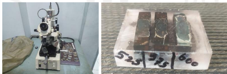
Gambar 3-10 Micro Vickers Hardness -M3 Microscope & Spesimen uji kekerasan
