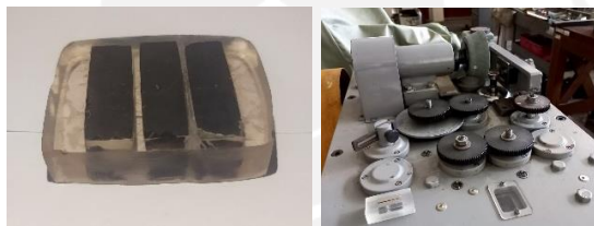
Gambar 3-11 Spesimen uji keausan dan Universal Friction Wear Tester
