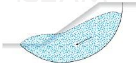
Figure 3.3 Slide Slope Failure Source: Das B.M., (1985)
