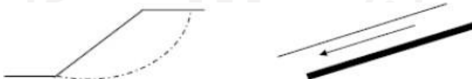
Figure 3.4 (a) Rotational slide and (b) Translational slide Source: Das B.M., (1985)
