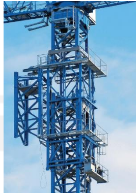
Gambar 3-4 Climbing Frame On Tower Crane Sumber : Google Image
