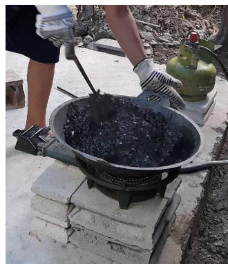
Gambar 12. Proses pelelehan plastik PP hitam
