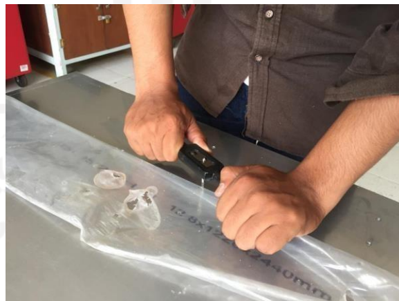
Gambar 4-22 Proses Tapping Manual
