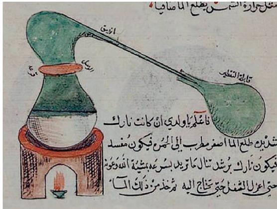
Gambar 1. 2 Destilasi “alembic” Jabir Ibn Hayyan abad ke 8 (Masic et al., 2017)
