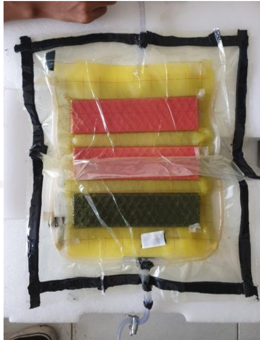
Gambar 3. 22 Proses Vacuum Infusion
