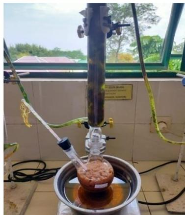
**Gambar 3. Proses Hidrolisis Sampel Batang Pisang**
