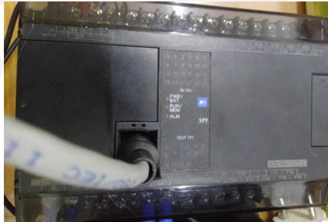
Gambar 3. 21 PLC Fuji NA0P40T-31C
