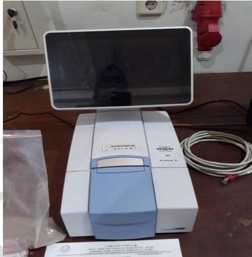
**Gambar 3.3.** *Fourier Transform Infra Red (FTIR)*
