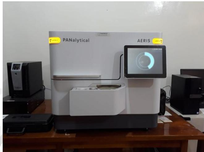
**Gambar 3.4.** *X-Ray Diffraction (XRD)*
