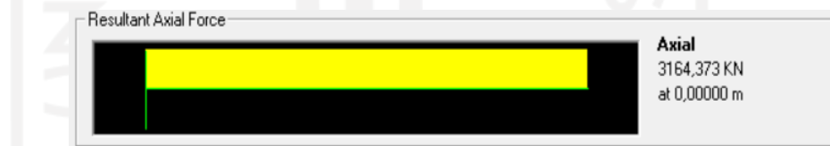
Gambar 5.29 Gaya Aksial Tarik Maksimum Batang Diagonal
