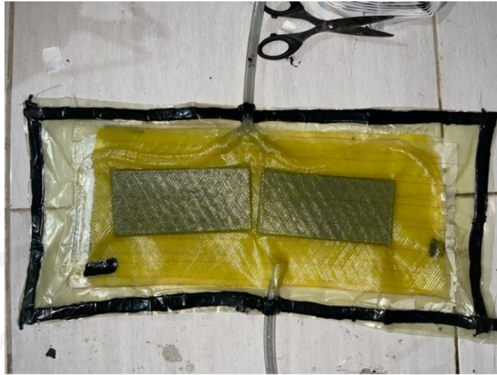
Gambar 3. 22 Proses Vacuum Infusion
