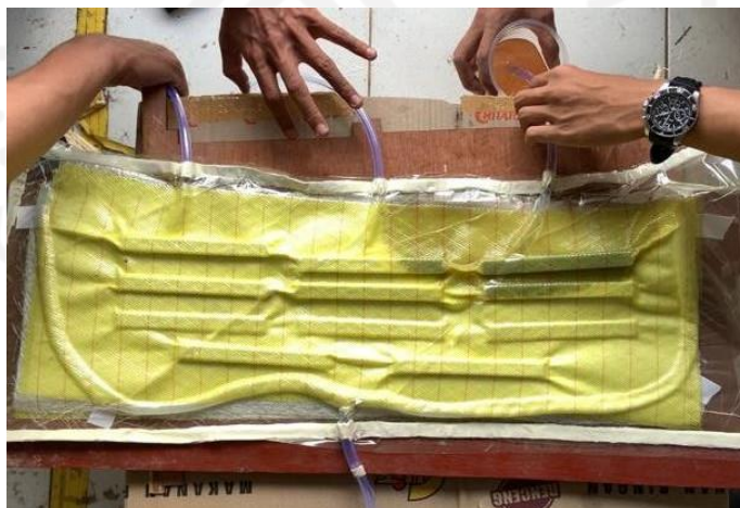
Gambar 3. 26 Proses Vacuum infusion
