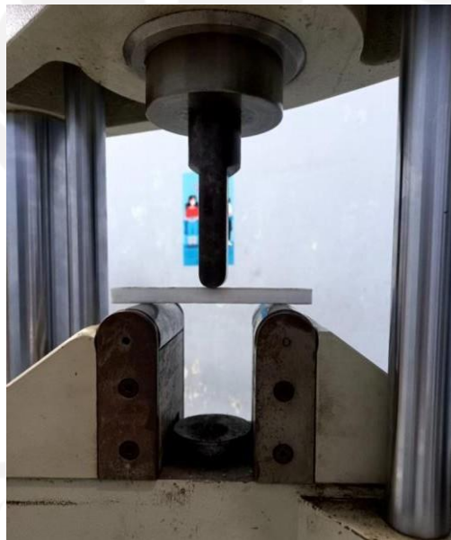
Gambar 4. 1 Proses Three Point Bending
