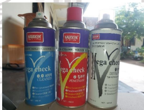
Gambar 3. 22 Peralatan Uji Dye Penetrant
