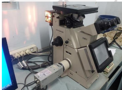
Gambar 3. 41 Mikroskop Metalurgi Olympus PME3
