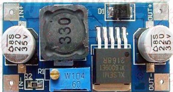
Gambar 3 - 15 DC to DC *Booster Converter*.
