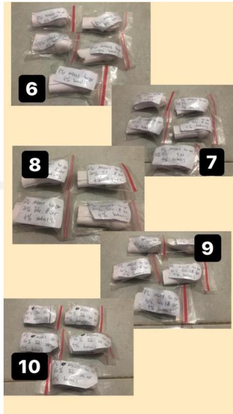
Gambar 4-12 Variasi Kulit Luar Silicone Rubber RTV M4503
