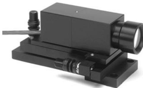
Gambar 2-16 *Autocollimator*
