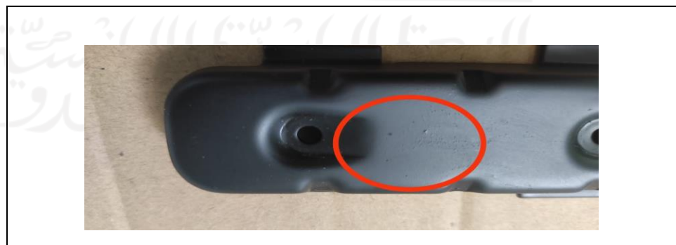
Gambar 4.16 Jenis defect dirty
