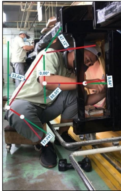
Gambar 4.7 Postur Pemasangan DC in Connector Cable
