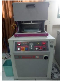
Gambar 3- 6 Mesin spin casting
