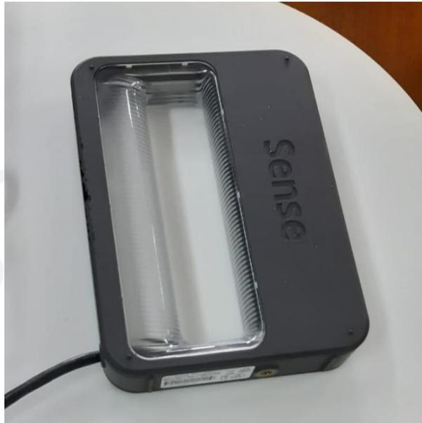
Gambar 3.7 Alat 3D Scan Sense
