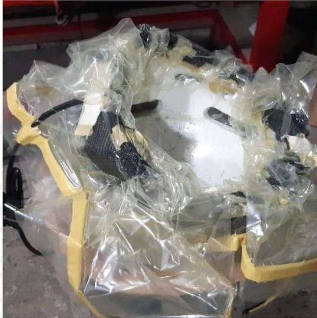
Gambar 4.7 Proses *Vacuum Infusion* Bagian Luar Helm Sepeda
