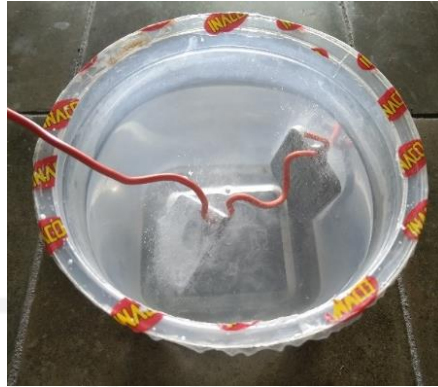
Gambar 3-14 Proses pencucian asam
