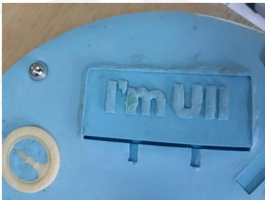
Gambar 4.7 Hasil vulkanisir silicone rubber benda dua
