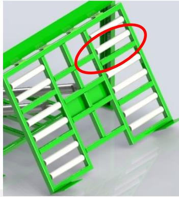
Gambar 4. 4 Roller Diameter 50 mm
