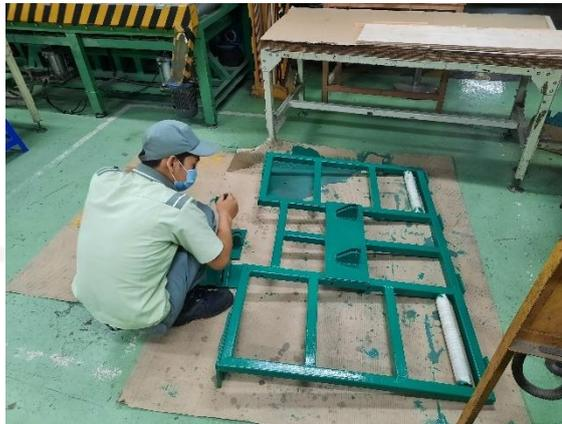
Gambar 4. 9 Proses *Painting Lifter Moulder Backpost*
