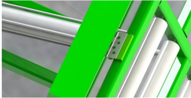
Gambar 4. 6 *Hinge* (Engsel)
