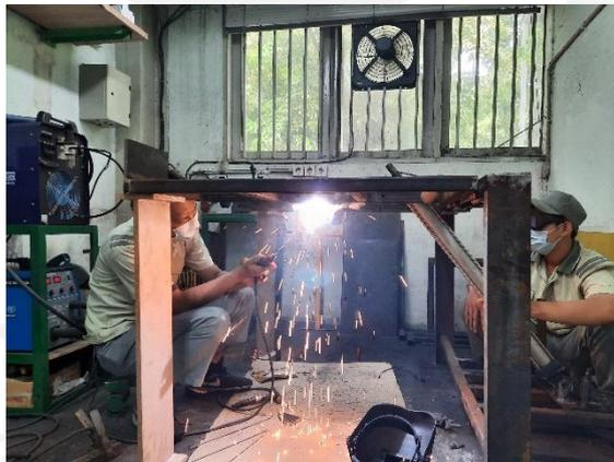
Gambar 4. 9 Proses Pengelasan *Lifter Moulder Backpost*
