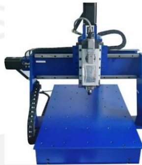
Gambar 3-15 Mesin Cedu CNC (3 Axis)
