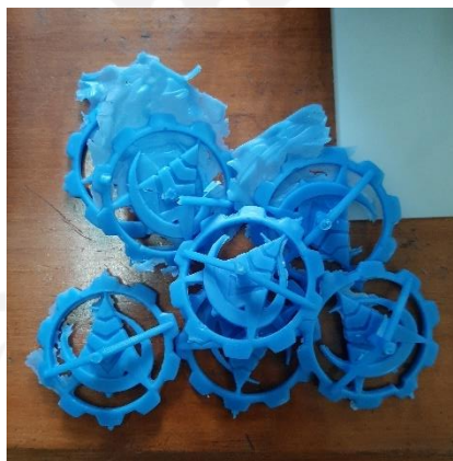
Gambar 4-12 Hasil Percobaan Model Lilin Gagal
