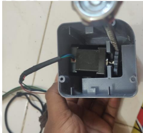
Gambar 4.13 Gear tertahan rack
