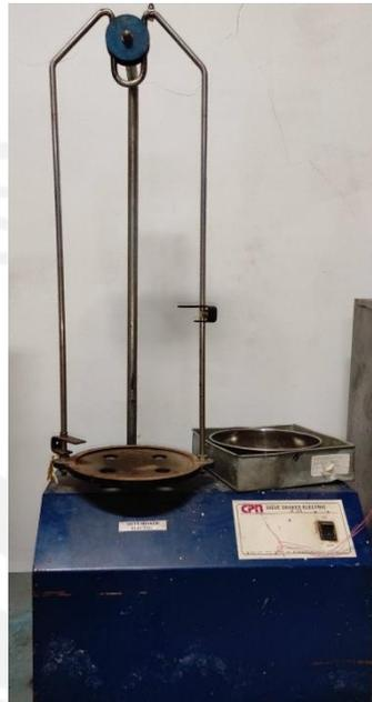
**Gambar L-1.1 Sieve Shaker Electric**
