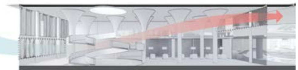
Cross ventilation by considering the direction of the wind source and the movement of hot air that tend to be upwards
