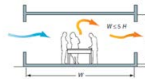
Figure 77. Passive Cooling Source: Author
