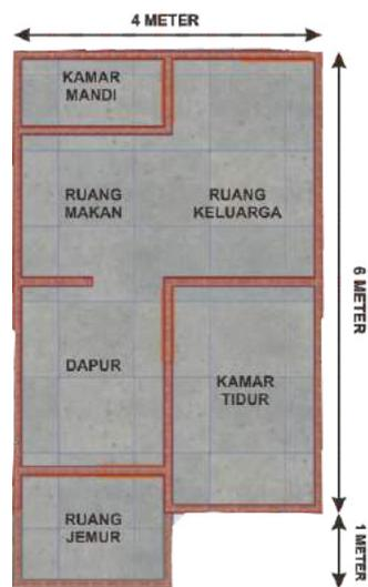
Gambar 66. Denah Hunian Tipe A 24 m<sup>2</sup>
