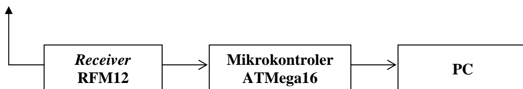
Gambar 3.2 Blok Diagram Penerima
