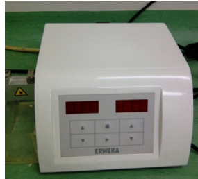
hardness tester (alat uji kekerasan tablet)
