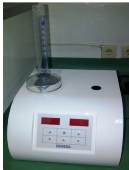
tapped density tester (alat uji pengetapan granul)
