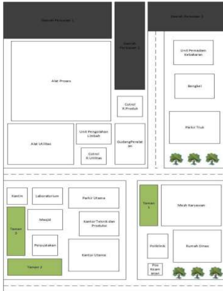
Gambar 4.2 Layout Pabrik Biodiesel
