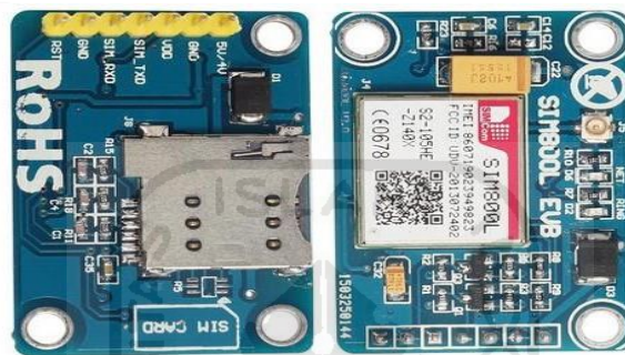
Gambar 2.5 GSM SIM 800v2
