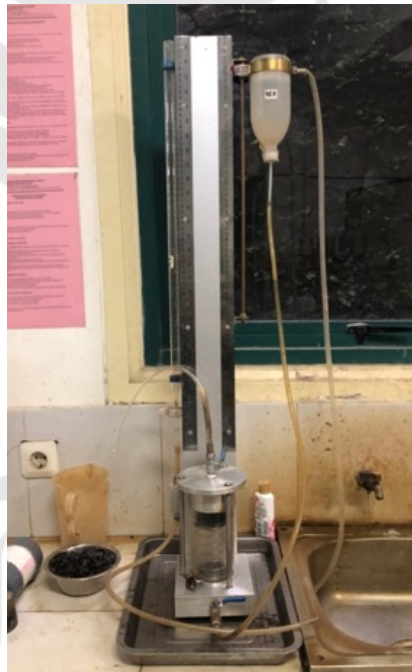
Gambar 5.6 Pengujian Constant Head Permeameter
