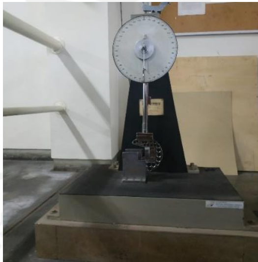
Gambar 3-17 Alat uji Impact Charpy
