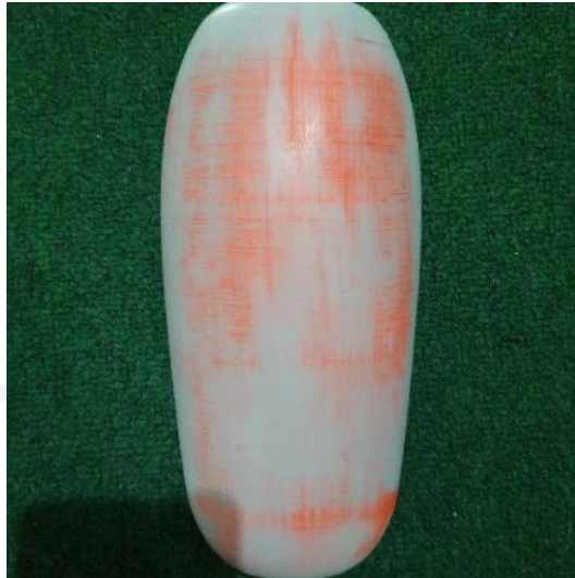
Gambar 4-15 Proses finishing master cetakan
