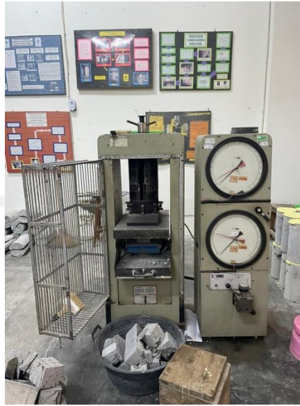
Gambar L-1.15 Compressing Testing Machine (CTM)
