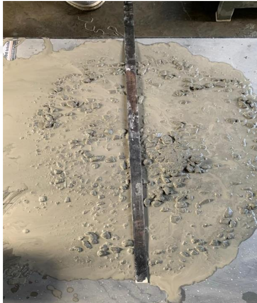
Gambar 5.9 Pengujian Slump Flow
