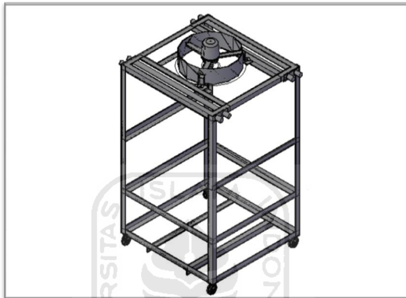
Gambar 3.5 Desain 3D kerangka dasar cooling tower
