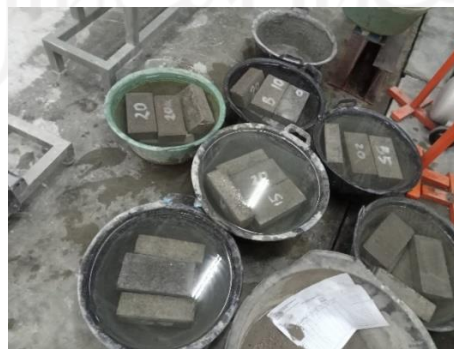
Gambar 4.3 Pengujian Daya Serap Air Paving Block
