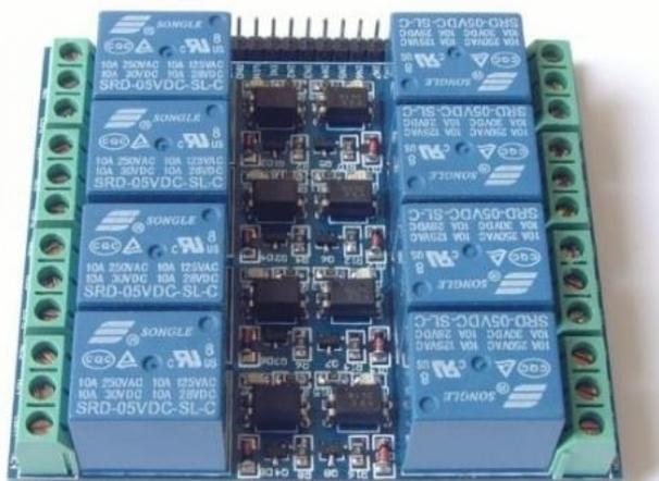
**Gambar 3.4 Relay 8-Channels**
