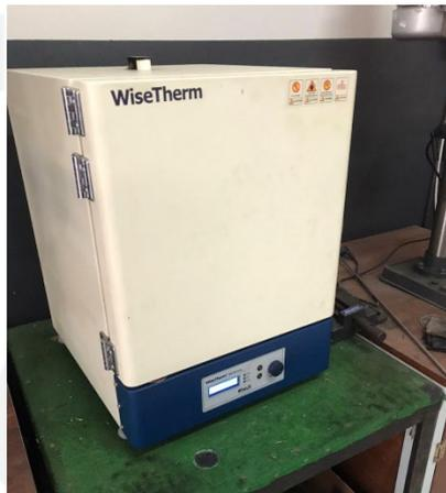
**Gambar 3- 4 Mesin Furnace WiseTherm**
