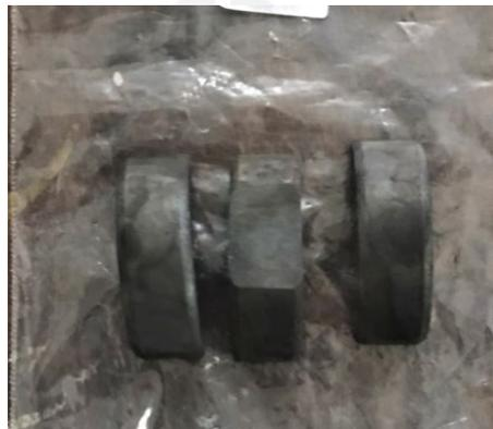
Gambar 4- 1 Bearing Hasil Proses Carburizing
