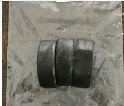
**Gambar 3- 7 Hasil Proses Carburizing**
