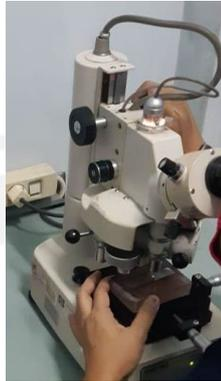
**Gambar 3- 10 Alat Uji Kekerasan Vickers Microhardness**
