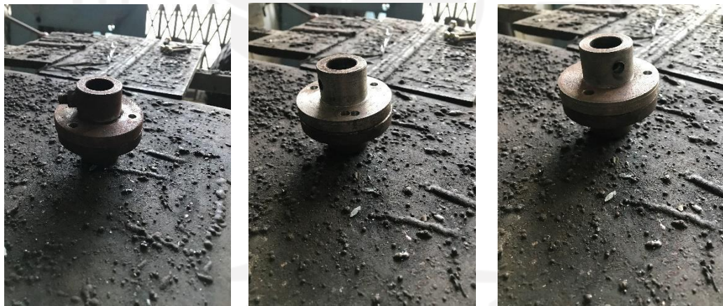
Gambar 4-4 Kopling normal (a), Kopling eksentrisitas 0,25mm (b), Kopling eksentrisitas 0,5mm (c)
