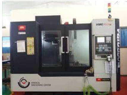
Gambar 3-3 Mesin CNC Roughing
