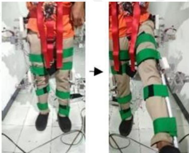
**Gambar 2.5** Prototipe Robot Rehabilitasi Kaki
