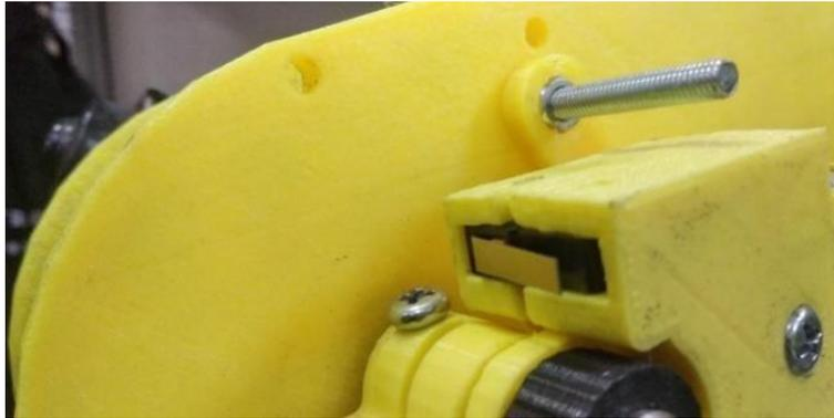
**Gambar 3.24** Posisi *Support Holder Limit Switch* Lutut
