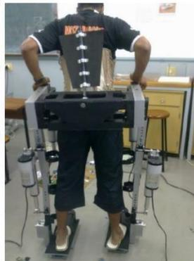
**Gambar 2.1** *Customizable Rehabilitation Lower Limb Exoskeleton System*
