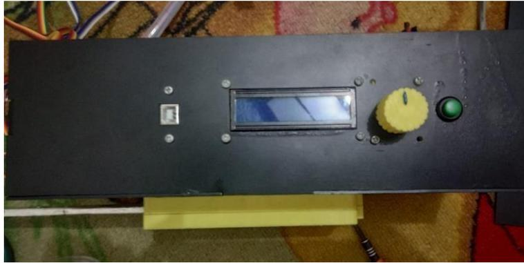
**Gambar 3.21** *Knop Rotary Encoder Menu*
