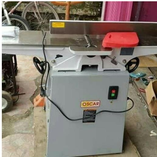
**Gambar 4- 4 mesin perata/jointer bambu**
