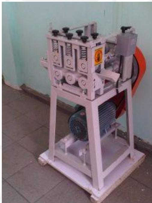
**Gambar 4- 3 mesin penipis bambu**
