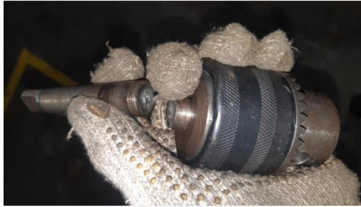
Gambar 4.2 Arbor Yang Mengalami Patah
