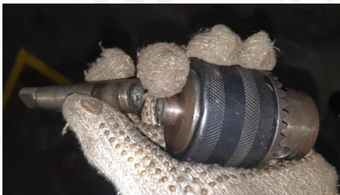
Gambar 4-2 : Arbor Yang Mengalami Patah
