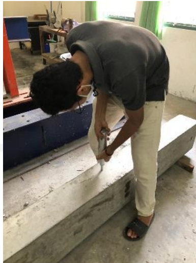
GAMBAR 29 HAMMER TEST SAMPEL BALOK
