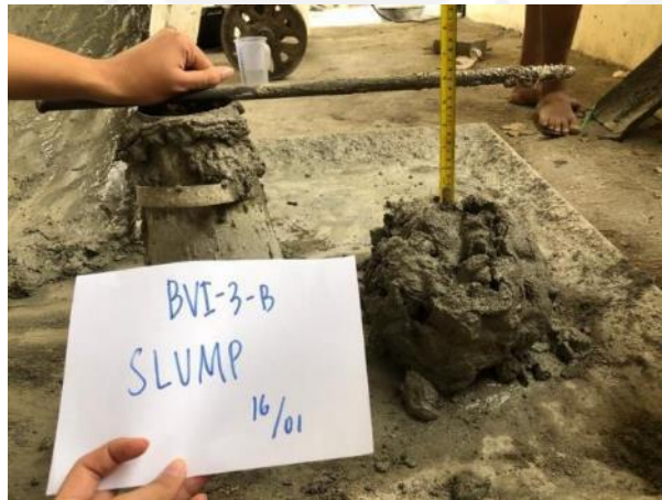
GAMBAR 18 SAMPEL NILAI SLUMP CAMPURAN BETON
