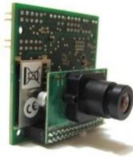
Gambar 2-8 Sensor Camera CMUcam3
